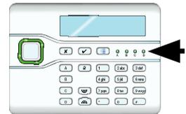
In a part setting system these LEDs glow to show you whether the system is set or unset. The left hand or ‘A’ LED glows when the system is full set, the other LEDs glow when the system is in one of the part set states.
